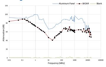
Test performed with a two-coat thickness.
