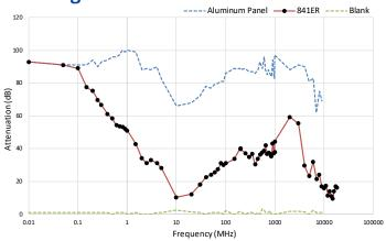
Test performed with a two-coat thickness.
