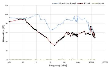
Test performed with a 2 coat thickness.
